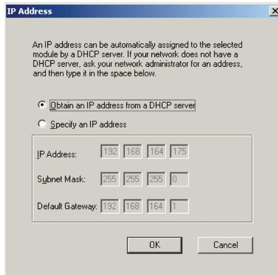
**Figure 2.12 – IP Address Screen – Attribution of the IP Address from DHCP Server**
